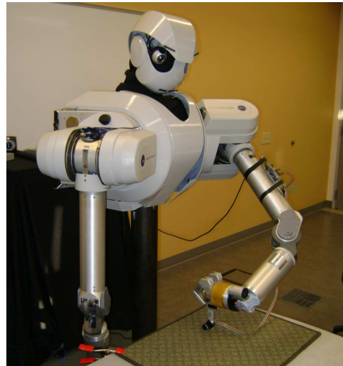
Fig. 1. Humanoid robot used in the experiments, which is shown here performing one of five scratching behaviors on a test surface.
