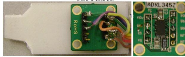
Left: the plastic fingernail with the attached accelerometer. Right: the other side of the accelerometer board (the ADXL345 is in the center).
