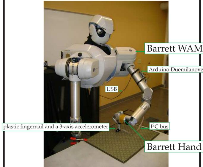
The accelerometer data was recorded at 400 Hz. With each surface the robot performed 10 trials. Each trial consisted of 5 scratches (3 lateral and 2 medial) executed at different velocities. Thus, the total number of behavioral interactions performed by the robot was  $21 \times 10 \times 5 = 1050$ .
